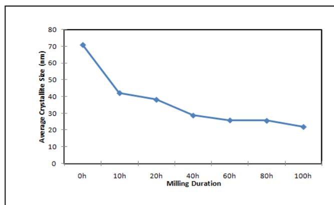
Fig. 2: Average crystallite size of Ti50%Al powder at various milling duration.
