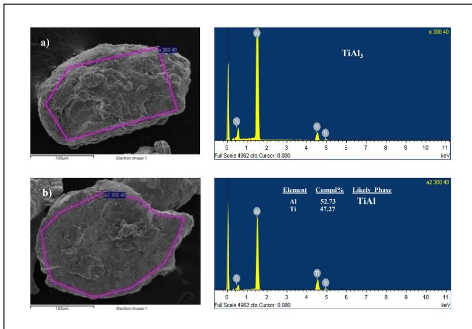
Fig. 3: FESEM image and EDX spectrum of Ti50%Al powder at 40h of milling duration with (a) TiAl<sub>3</sub> and (b) TiAl phase.
