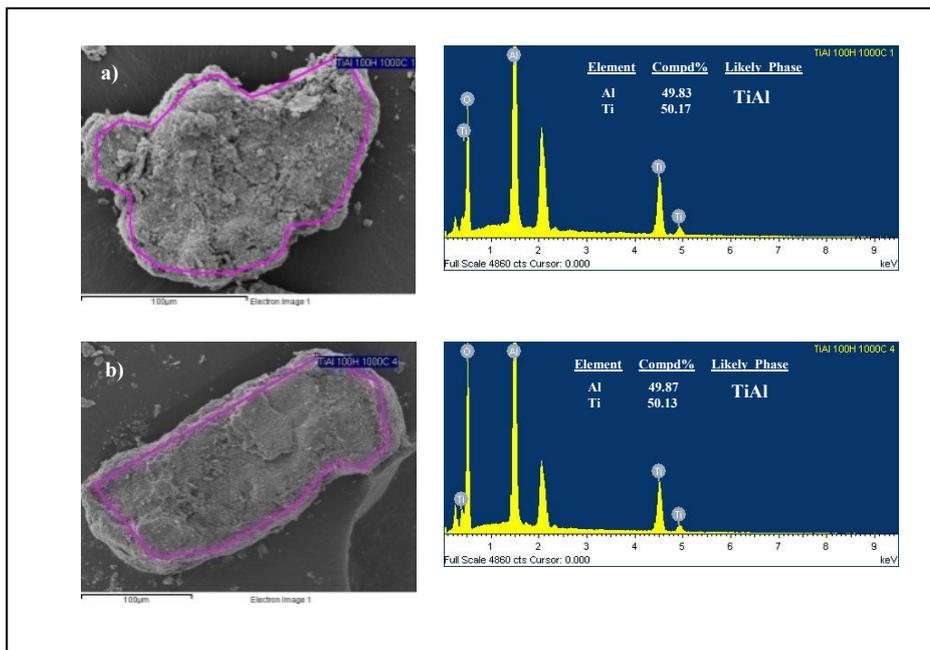
Fig. 7: FESEM image and EDX spectrum of Ti50%Al powder at 100h of milling duration with TiAl phase.
