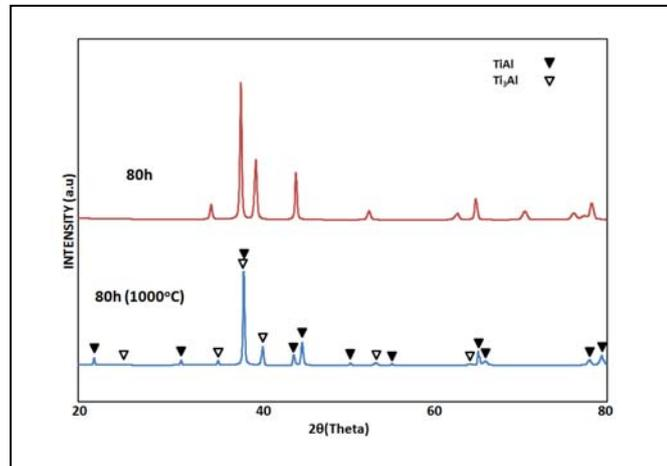
Fig. 5: X-ray spectrum of 80h milled Ti50%Al powders before and after heat treatment.
