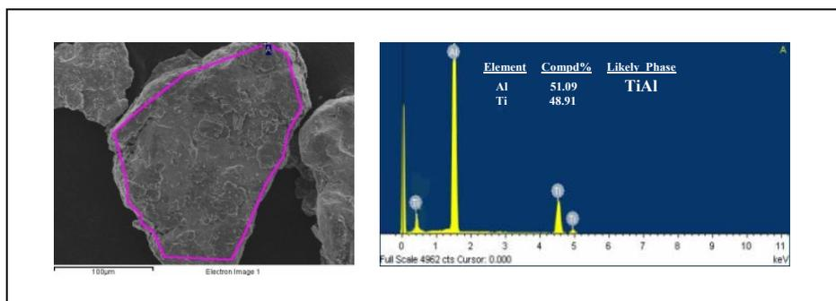
Fig. 4: FESEM image and EDX spectrum of Ti50%Al powder at 100 h of milling duration with TiAl phase.
