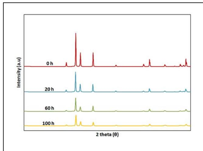
Fig. 1: X-ray spectrum of Ti50%Al powders at various milling duration.
