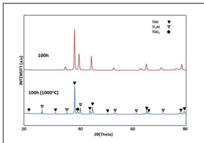
Fig. 6: X-ray spectrum of 100h milled Ti50%Al powders before and after heat treatment.
